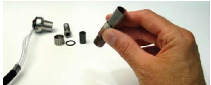
Completely disassemble the handpiece. The two main components you will be servicing are the barrel, which has a precision bore for the piston, and the piston itself.
